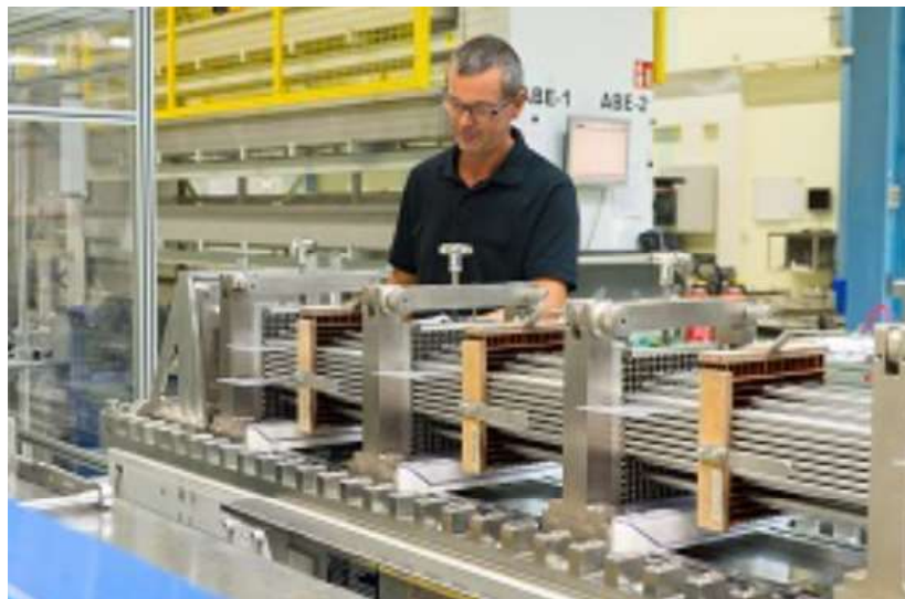
Figure 3.3.4-2. Workbench for assembling fuel assemblies in the Lingen fuel factory of Framatome (Germany)
