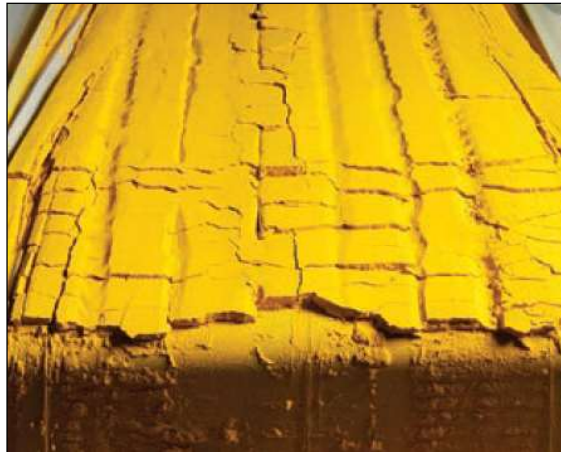
Figure 3.3.1-7. – Yellowcake on the production line
