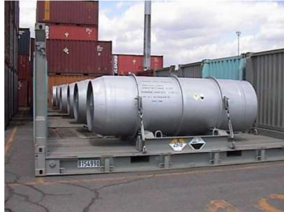
Figure 3.3.2-2. UF_6 transport cylinders on their way to the enrichment plant
