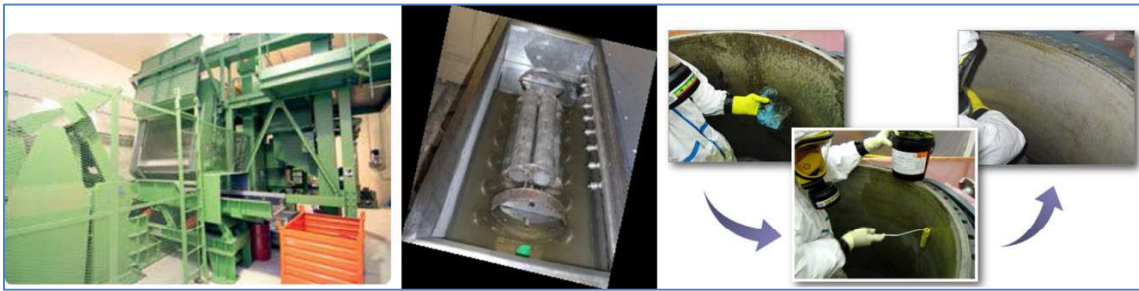
Figure 3.3.7-5. – Surface decontamination techniques for metallic items, from left to right: abrasive blasting unit, ultrasound bath and application of gel
