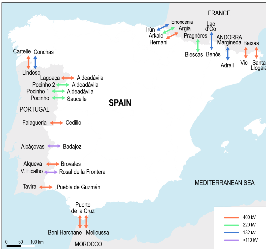
Figure 7.4 Spain's current interconnections with neighbouring countries
